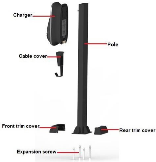
Figure A-10 Floor standing assembly drawing
