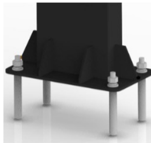
Figure A-15 Fixed column
